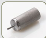
11-1414 Solvent Filter 10µm SS with 1/16" Stem
